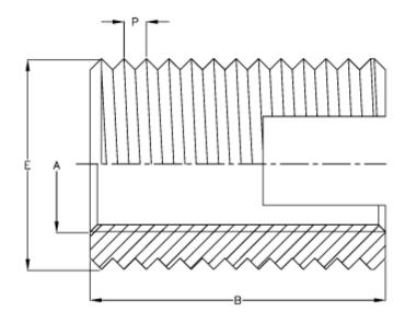
Female thread A = M20 Length B = 27 Male thread E = 26.0 Min hole depth blind hole = 32
